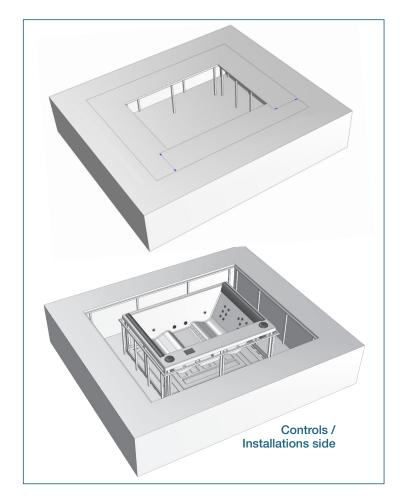
NB: Make sure the weight is supported on the base and not on the edges.
